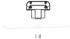
1. To insert the connector into the base and put the sheet iron on the connector, then fix them by screws.
